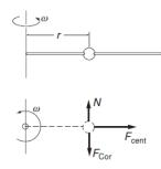
In the rotating frame, the pseudo forces are: centrifugal force  $F_{cent}$  and Coriolis force  $F_{Cor}$ , as shown. N is the reaction force applied by the rod on the bead. It is obvious, that in the non-inertial frame, on which we use plane polar coordinates, we obtain
